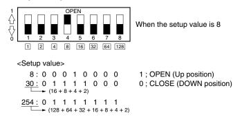
When the switch S703-6 is set to CLOSE (DOWN position), this switch is used for the IP address when connected to the DATA LAN and is fixed to "10.64.5.1".
